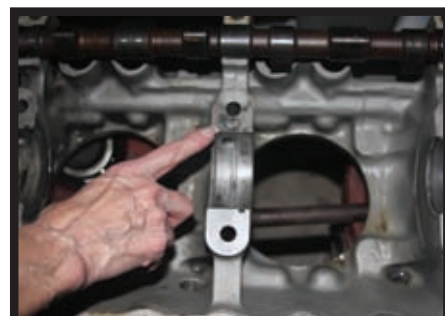
10. Lyc. Engine Case "Fretting" example
