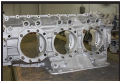
8. Latest series case (Notice heavier webbing between cyls.)
