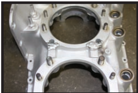
7. Lyc. Case welded between cyls. Typical cracking area between cyls.
