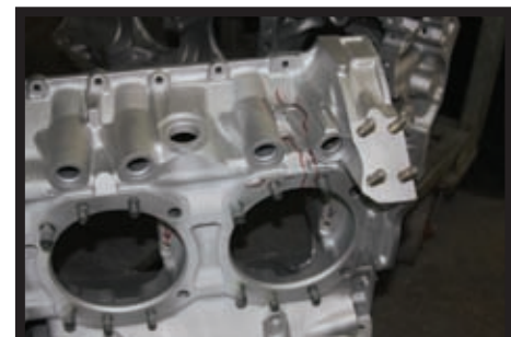
4. Lyc. Case with 8hrs. SOH, connecting rod bolts came lose and rod came thru case
