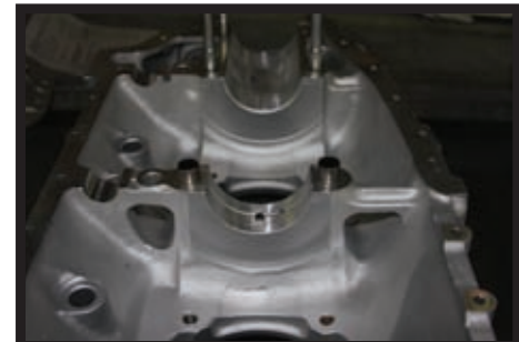
5. Lyc. Case with thru-hole sleeves
