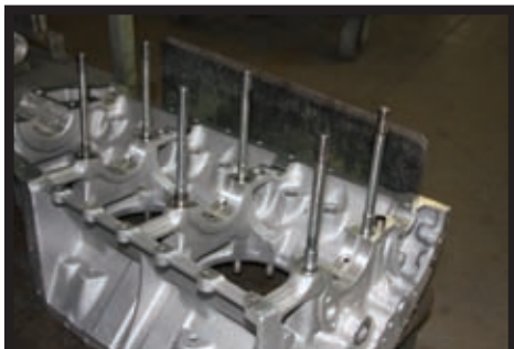
6. Lyc. Case with thru-bolts & hole sleeves
