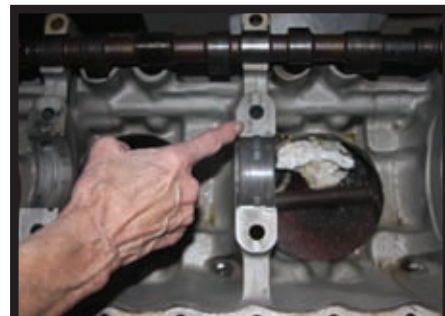
11. Lyc. Engine Case "Fretting" example
