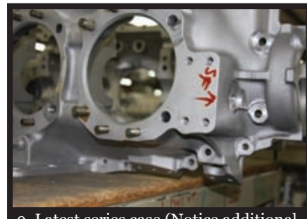
9. Latest series case (Notice additional bolt hole on lower row.) Older cases have 2 holes not 3
